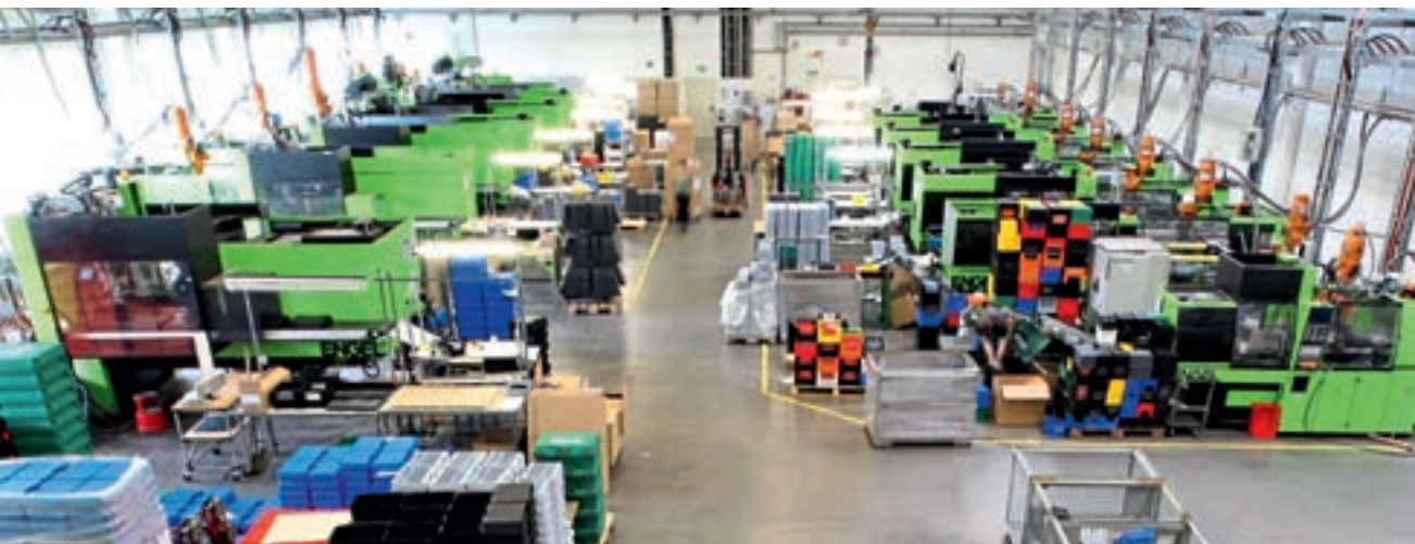
A look into injection moulding production: W.AG manufactures three million plastic cases each year.
