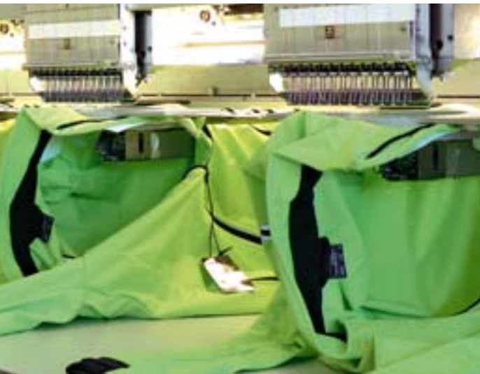
Precise and fast: efficient embroidery machines finish textiles and caps. Daiber was one of the first companies to offer professional textile finishing on a grand scale.
